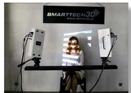
Integrated system of two 3D scanners allows us to make a measurement from different angles
