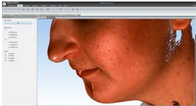
Cloud of points with XYZ coordinates and RGB color - raw scanned data
