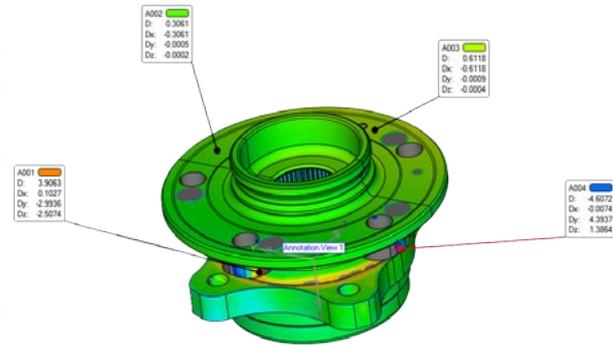
The scanner is available in three basic resolutions: 2x5 MP, 2x9 MP, and 2x20 MP for application that focus on high detail representation. The system can be additionally equipped with a set of exchangeable lenses, allowing a customer to change the scanning volume and adapt to different dimensions or complexity of scanning details.
