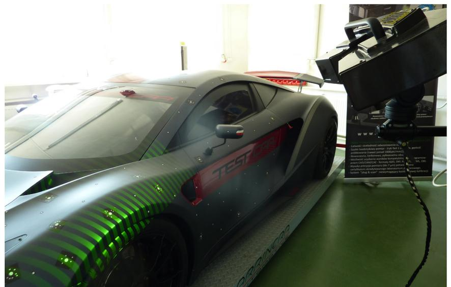
MICRON3D green stereo is a professional, factory-calibrated metrology tool, certified by the manufacturer according to the German VDI / VDE 2634 standard, and its measurement accuracy can be additionally confirmed by a certificate of an independent accredited metrology laboratory.
