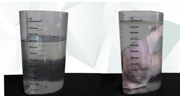
*Determining the volume of an object based on changes in the height of the liquid column*
