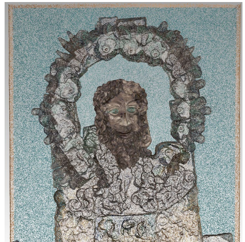
Point cloud combining data from photogrammetry and 3D scanner
